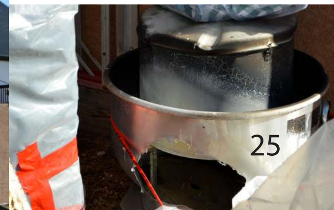
"The fire was so hot it blew out the side of the fan. This is stainless steel." O'Malley's owner Jeff Hulsmann points out the damage. The fire was hot enough to melt through the side of one of the stainless steel exhaust fans above the kitchen.
